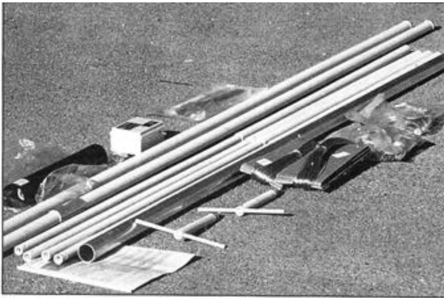
small-antenna test mast. The combination of aluminum boom, copper wire, and white fiberglass supports creates an unusual first impression, compared to more common antenna types.
