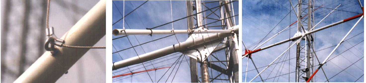
The loop wires are fixed on the fiberglass tubes by us in our factory
