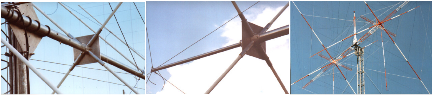
The loop wires are fixed on the fiberglass tubes by us in our factory
